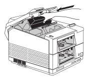
4 Grasp the tab protruding from the left side of the cartridge and flex it to break it loose.
